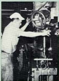
Tom Lopez, Machine Shop, was employed by Bell-Band before coming here in October, 1950. He left to serve in the Navy from September, 1951 until September, 1953, when he returned. Tom usually operates a Radial Drill. In this picture he is working on a bearing housing for a Slew Roll machine. Tom likes to hunt and fish and enjoys watching football and basketball. He belongs to the Veterans of Foreign Wars, an which organization he is quite active.
